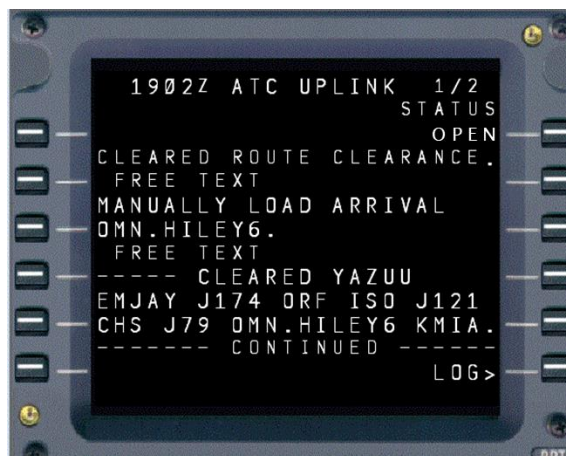
Figure 24. Clearance Uplink with Free Text Arrival – DAT Code 1FANSER2PDC or FANSER Example
