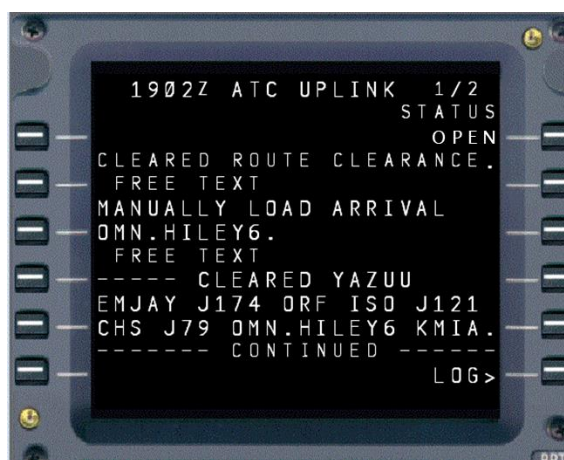
Figure 26. Clearance Uplink with Free Text Arrival – DAT Code 1FANSER2PDC or FANSER Example
