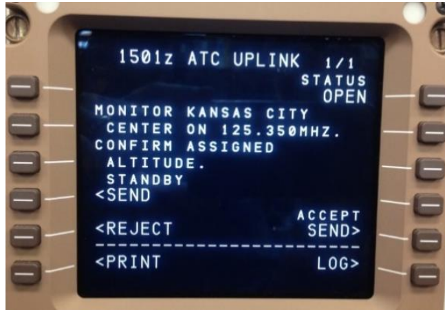
Figure 20. CPDLC Monitor Message with Confirm Assigned Altitude
